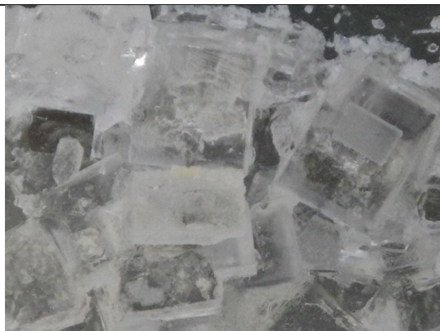
Taking an even closer look at the salt crystals. Note the cubic crystal habit
